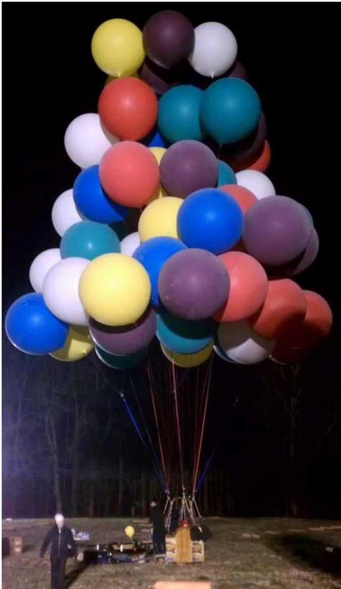
on the balloons, as they were inflated across the airfield. This concerned me; we've never flown when the cells were this cold. Would the balloons become brittle in the cold? When we assembled the cluster, the balloons banged into each other, shearing off some of the ice and creating a very localized snowfall. They did not, however, pop or shatter.
